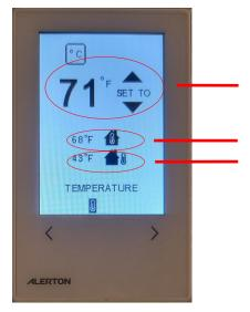
Desired Temp Set Point Use the up or down arrows to adjust the temp between 70°-74° in most cases.
